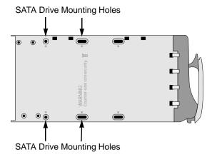
Figure 10.M500f/i/p drive carrier mounting holes
